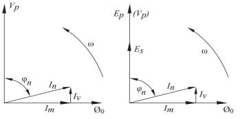
Fig. 16-2: Vector diagram of no-load transformer
