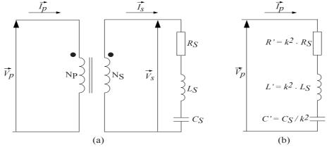
Fig. 16-7: Ideal transformer, loaded with a series R-L-C circuit: impedance transformation
