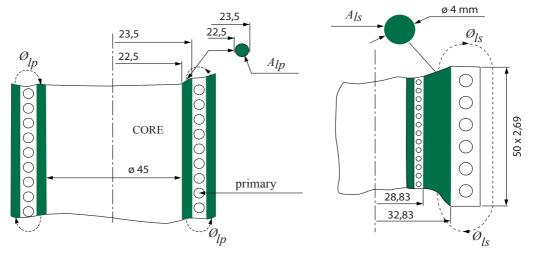
Fig. 16-10a: Primary leakage flux of transformer in fig. 16-8a
