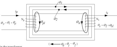
Fig. 16-4: Fluxes in the transformer
