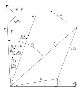
Fig. 16-6: Vector diagram of transformer with inductive load
