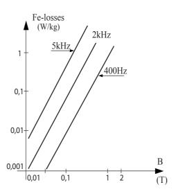
Fig. 16-12: Iron losses with the frequency as a parameter
