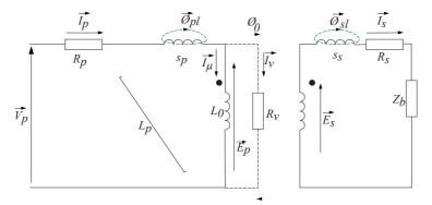
Fig. 16-5: Transformer with losses and secondary load
