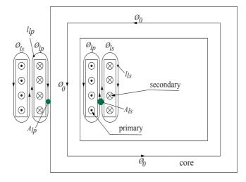
Fig. 16-9: Leakage fluxes by a coaxially wound transformer
