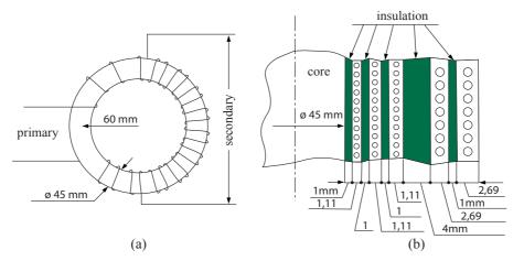
Fig. 16-8: Ring core transformer (a) cross-section (b) core and windings
